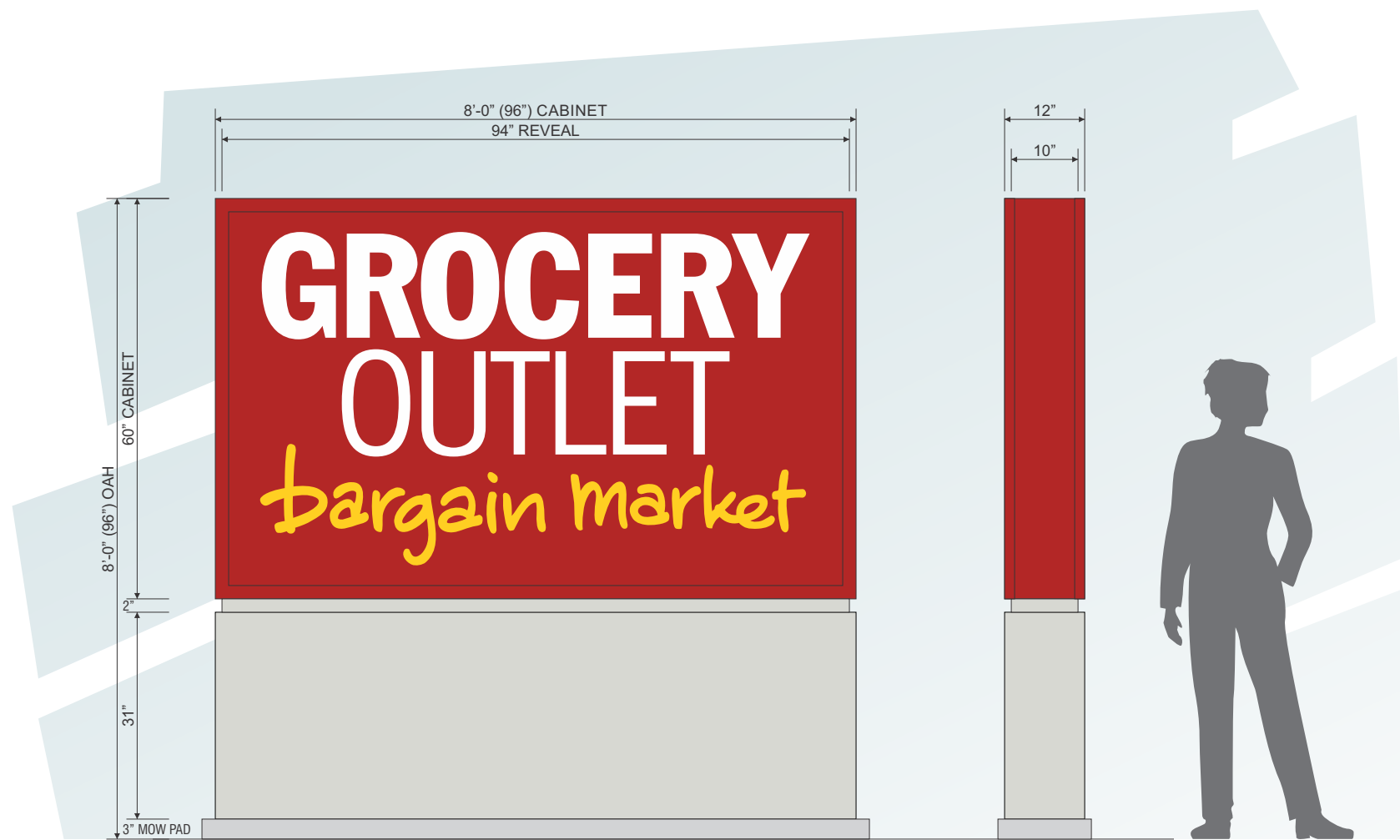
2 PROPOSED : D/F INTERNALLY ILLUMINATED MONUMENT SIGN CABINET / STRUCTURE ( 1 ) REQUIRED
