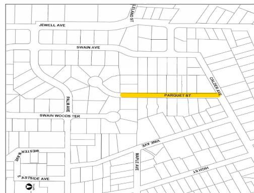
**DESCRIPTION:** Replacement of approximately 850 lineal feet of 6-inch sewer main on Parquet Street. This work includes slurry seal of Parquet Street that is affected by the sewer line replacement work. The work was constructed with the Parquet Street Water Main Replacement project #0818-20.09.
