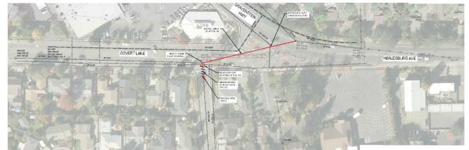
**DESCRIPTION:** Reduce flows to the Zimpher Creek sewer main by rerouting the flows from Covert Lane to Healdsburg Avenue. The project consists of a new 8-inch sewer, approximately 250 LF, which allows for gravity flow. The next step is to update the cost estimate for the following year's construction.
