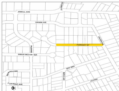
**DESCRIPTION:** Replace approximately 800 lineal feet of 6-inch water line on Parquet Street. This work includes slurry seal of Parquet Street that is affected by the water line replacement work. The work was constructed with the Parquet Street Sewer Line Replacement project #0615-21.01.
