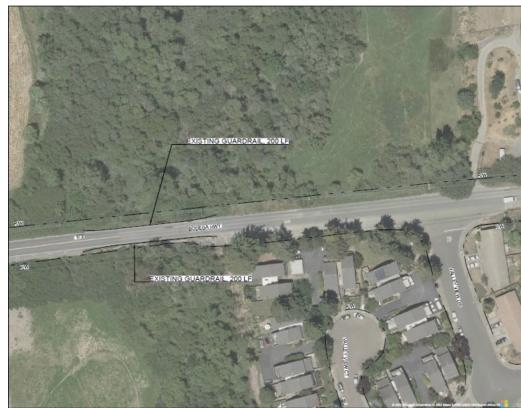
**DESCRIPTION:** Remove existing bridge guardrail and replace approximately 765 lineal feet of guard rail. Work includes replacing signage and related appurtenances. This project is primarily funded with a Highway Safety Improvement Program (HSIP Cycle 11) grant from the State.
