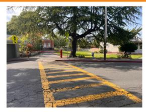
**DESCRIPTION:** Taft Street/Sunset Avenue – upgrade crosswalk markings including advanced yield markings and install double-sided flashing pedestrian crossing signs with circular LED beacons in similar style to other Sebastopol crossings. Install advanced pedestrian crossing signage. Upgrade curb ramps to comply with current ADA standards. Install edge line striping for traffic calming on Sunset Avenue between Taft Street and Johnson Street
