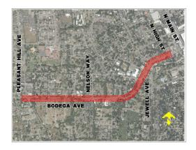
**DESCRIPTION:** Bodega Avenue project design which includes preliminary and final design, geotechnical engineering, project management, and environmental documentation (CEQA/NEPA). This work is the design phase for the Bodega Avenue repaving construction (project nos. 0512-74.08 and 0513-74.09).
