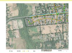
**DESCRIPTION:** This project will update the 2005 Sewer System Master Plan. The plan will include system capacity analysis and identify deficiencies in sewer system that could result in sewer overflows. The master plan will identify a Capital Improvement Program to upgrade system deficiencies and will include maintenance repair and replacement projects identified in Public Works' ongoing CCTV investigations.
