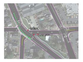
**DESCRIPTION:** The project is the modification of Palm Avenue to one-way (westbound) traffic from Petaluma Avenue to S. Main Street. The work includes installation of sidewalk on the north side of Palm Avenue, a street overlay, and signage and markings. The project was designed and was not approved to move forward by Council on 3/7/23.
