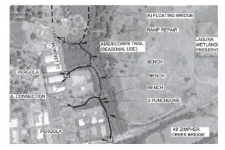
**DESCRIPTION:** This trail extension project located in the Laguna Wetlands Preserve from the Sebastopol Lift Station to Sebastopol Avenue. Design and CEQA review are complete and the construction bid documents are being prepared. The project consists of constructing a trail extension, a pedestrian bridge at Zimpher Creek, improvements to the current trail segments, addition of some benches, addition of trail signs, and a rail entry south of the Community Center parking lot.
