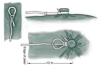
Figure 11: Plastic Tie-Down Buttons
