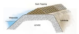
Figure 3: Sack topping on a levee
