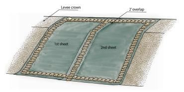
Figure 14: Emergency spillway using plastic sheeting and sandbags
