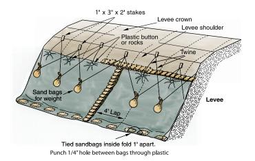
Figure 10: Wavewash Protection
