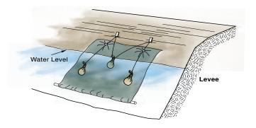
Figure 9: Waterside boil protection
