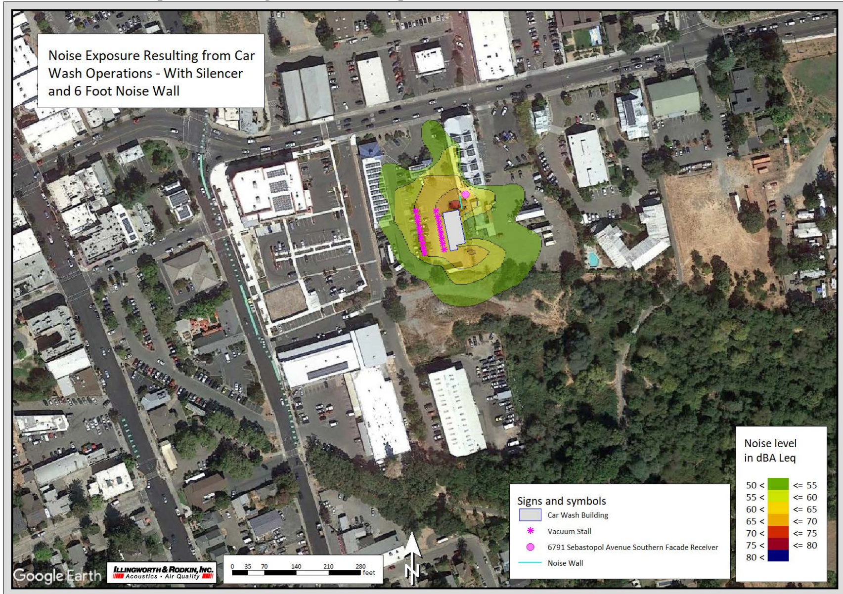
FIGURE 6 Noise Exposure Resulting from Car Wash Operations – With Silencer and 6ft Noise Wall
