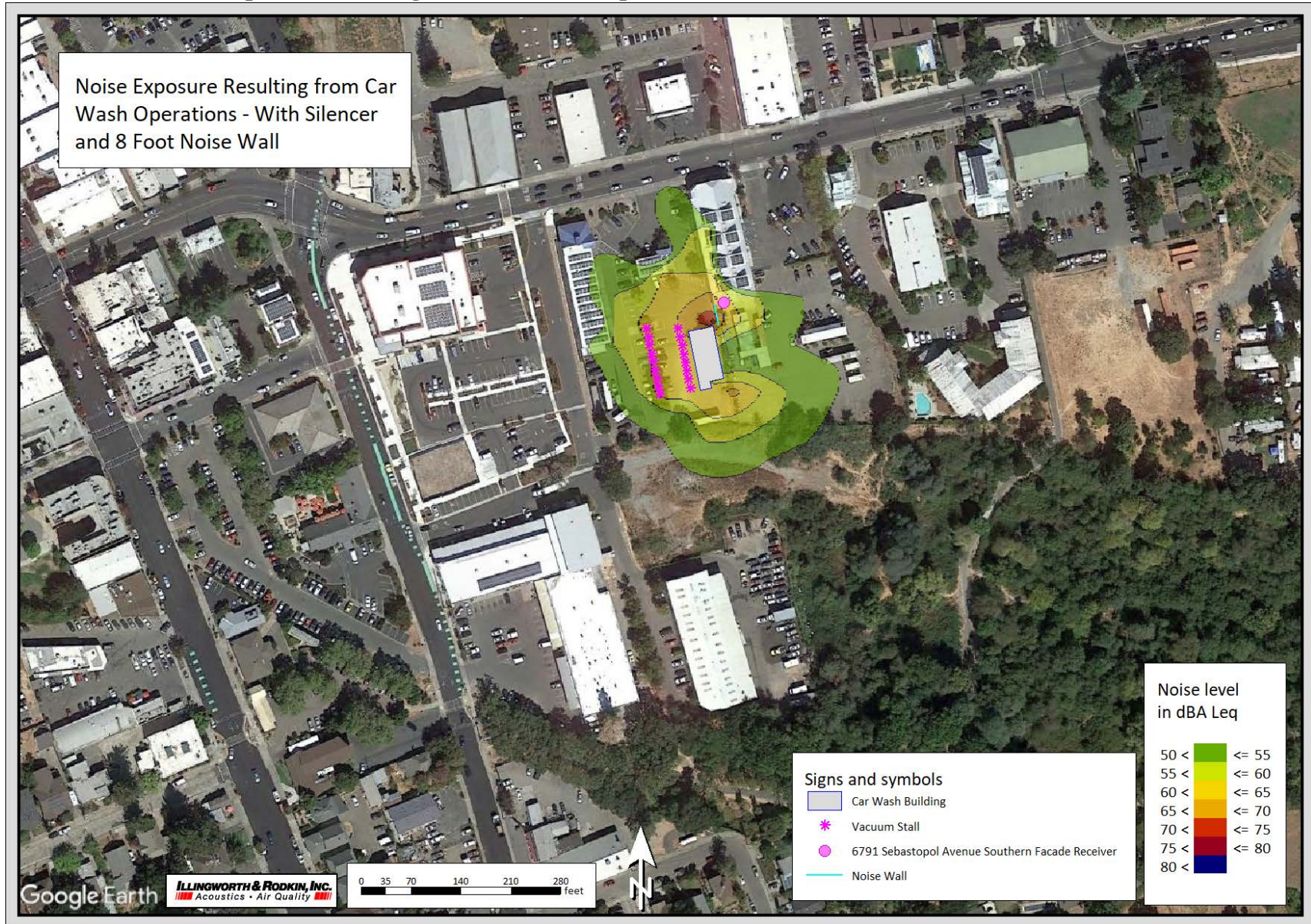
FIGURE 7 Noise Exposure Resulting from Car Wash Operations – With Silencer and 8ft Noise Wall
