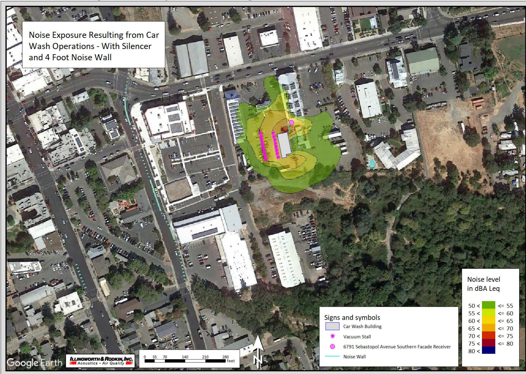
FIGURE 5 Noise Exposure Resulting from Car Wash Operations – With Silencer and 4ft Noise Wall
