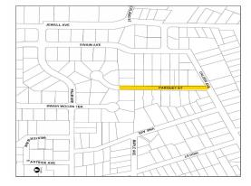
**DESCRIPTION:** Replacement of approximately 850 lineal feet of 6-inch sewer main on Parquet Street. This work includes slurry seal of Parquet Street that is affected by the sewer line replacement work. The work is being completed with the Parquet Street Water Main Replacement project #0818-20.09
