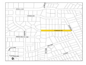
**DESCRIPTION:** Replace approximately 800 lineal feet of 6-inch water line on Parquet Street. This work includes slurry seal of Parquet Street that is affected by the water line replacement work. The work is being completed with the Parquet Street Sewer Line Replacement project #0615-21.01).
