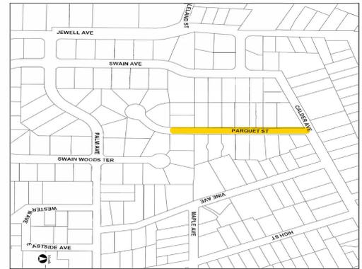
**DESCRIPTION:** Replace approximately 800 lineal feet of 6-inch water line on Parquet Street. This work includes slurry seal of Parquet Street that is affected by the water line replacement work. The work is being completed with the Parquet Street Sewer Line Replacement project #0615-21.01).
