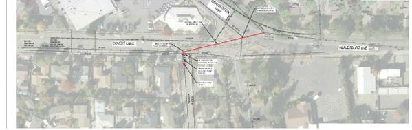
**DESCRIPTION:** Reduce flows to the Zimpher Creek sewer main by rerouting the flows from Covert Lane to Healdsburg Avenue. The project consists of a new 8-inch sewer, approximately 250 LF, which allows for gravity flow.
